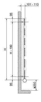
(\*) Pipe center (I) measure of the fixing kit
